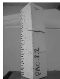
fig. 3. Fracture development in PAC mortar after the capillarity essay.
